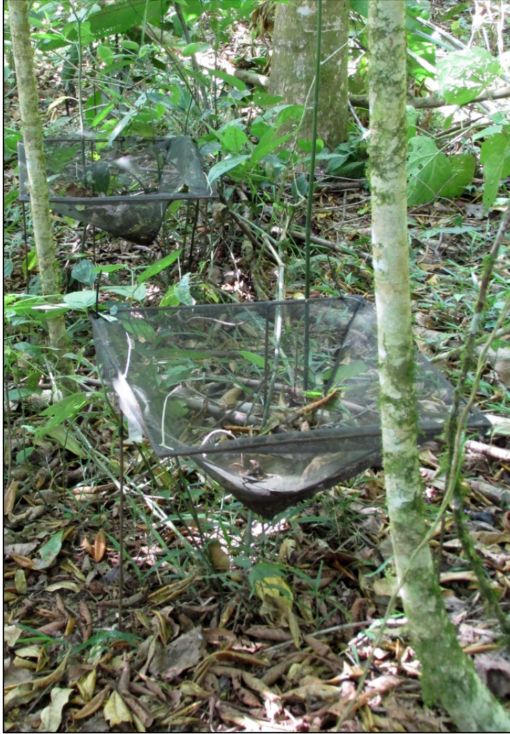
FIG. A2. Seed traps in a restoration site at Las Cruces Biological Station, Costa Rica. Traps were 0.25 \text{ m}^2 with a frame made from soldered rebar and a sheet of cut and sewn fiberglass window screening connected to the frame with plastic zip ties. The aperture of the fiberglass window screening was 0.69 \text{ mm} . Pocket depth was 30 \text{ cm} . The rim was 55 \text{ cm} above the ground. Photo Credit: J. Leighton Reid.
